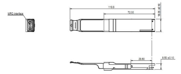
Attention: To minimize MPO connection induced reflections, an MPO receptacle with 8-degree angled end-face is utilized for this product. A female MPO connector with 8-degree end-face should be used with this product as illustrated in Figure 5.
